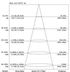
Note:The illu Curves indicate the illuminated area and the average umination when the luminaire is at different distance.
